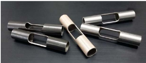
Fig. 4. Fabricated specimens from the unirradiated fuel claddings by using the laser cutting machine.
