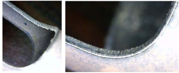
Fig. 5. Cutting details of the fabricated specimen with thick oxide by using the laser cutting machine.
