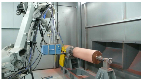
Fig. 2. Cold spray coating of a medium-size canister.
