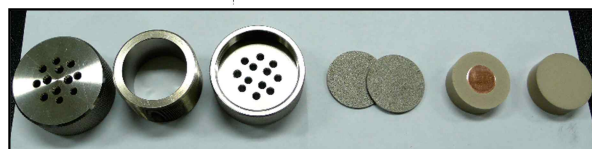
Fig. 4. Corrosion cell in a simulated environment.
