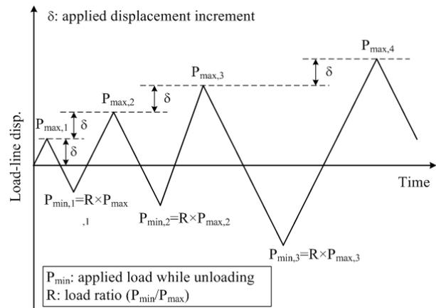
Fig. 1 Cyclic loading sequence applied for cyclic J-R fracture toughness tests
