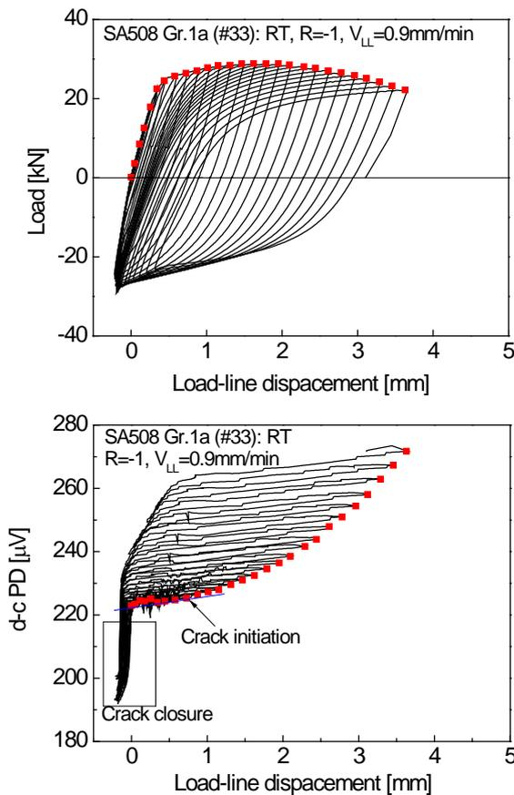
Fig. 2 Sample data of cycle J-R fracture toughness test
