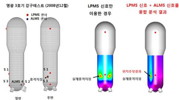
Fig. 2 Integrated Analysis of LPMS & ALMS signals for estimating the Impact location
