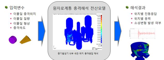
Fig.4 Numerical Simulation of Impact Response of Pressurized Vessel due to Foreign-Object
