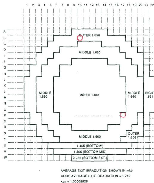
Fig. 1. Position of DI Test Channel and Exit Irradiation
