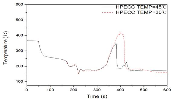
Fig. 5. Temperature of the Fuel Sheath
