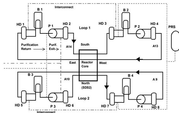
Fig. 1. CANDU Simplified Circuit Diagram
