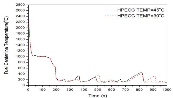
Fig. 3. Temperature of the Fuel Centerline
