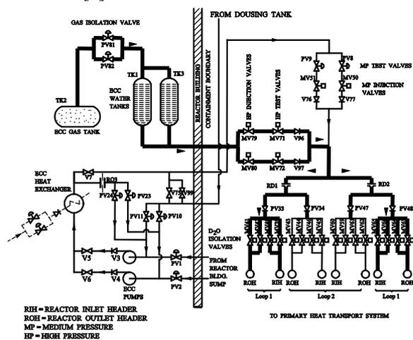
Fig. 2. ECC System Simplified Diagram
