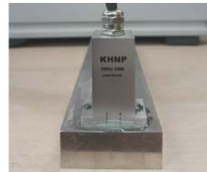
Fig. 6. PA probe and stainless steel specimen
