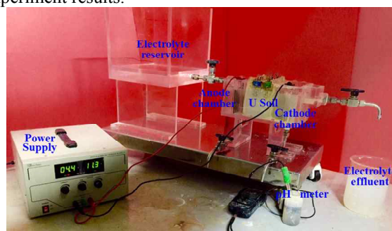
Fig. 1. Laboratory electrokinetic decontamination equipment manufactured for experiment
