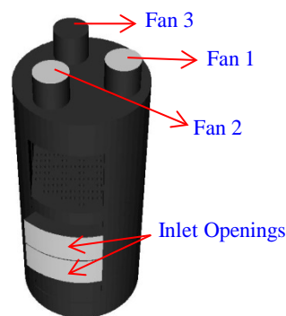
Fig. 4. Inlet Openings and Fan Outlets
