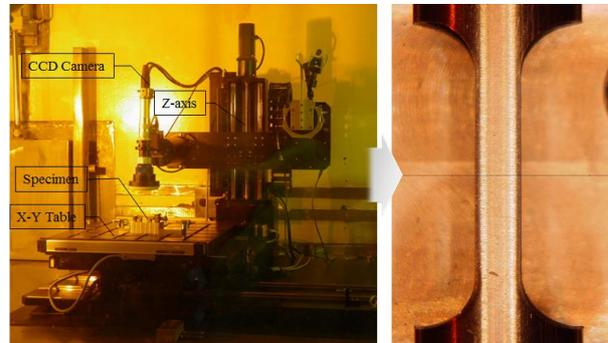
Fig. 2. Dimensional measurement set-up in a hot cell and the image of the specimen during the measurement.
