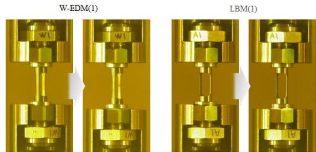
Fig. 5. Deformation behavior of the specimens at the initial and final status of the tensile tests.
