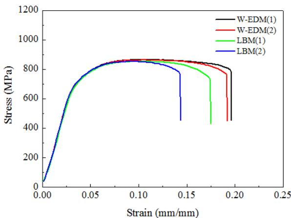
Fig. 4. Stress-strain curves for the tensile tests of the axial tensile specimens depending on the processing type.
