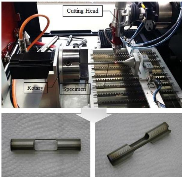
Fig. 1. Laser cutting system and fabrication of the tensile testing specimens from the unirradiated fuel cladding.
