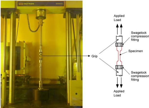
Fig. 3. Experimental set-up and schematic illustration for the tensile testing of the tube specimen in a hot cell.
