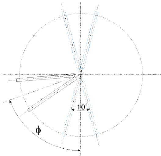
Fig. 1. Angle of rotation of V-shape tube bundle.
