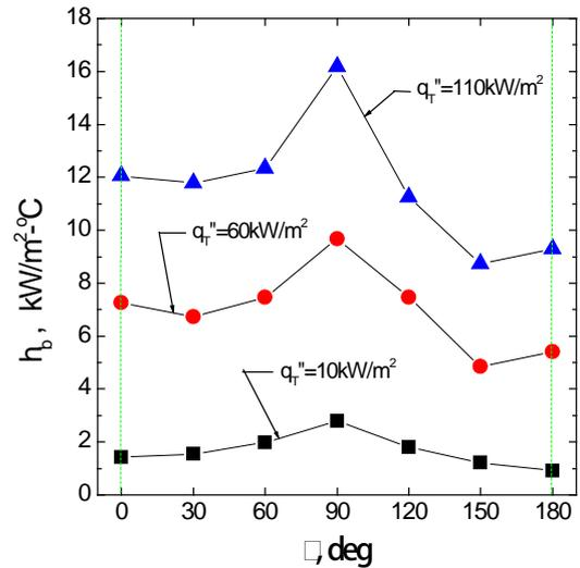
Fig. 4. Variations in heat transfer coefficient as rotation of angle changes.
