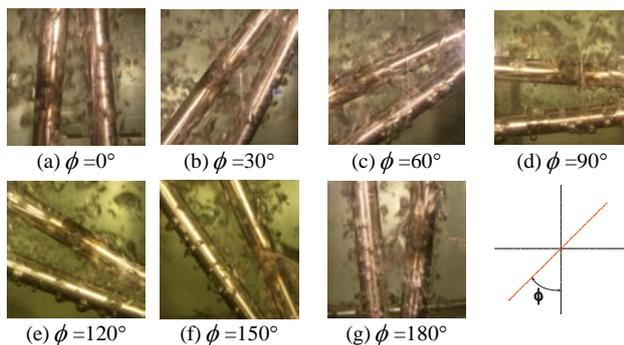
Fig. 5. Photos of pool boiling at  $q_T'' = 60 \text{ kW/m}^2$ .
