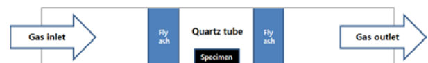
Figure 3. The diffusion test apparatus system. A picture of real apparatus (top) and the schematic (bottom)
