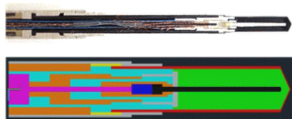
Fig. 2. A Farmer-type ion-chamber (PTW N30013) was divided into two pieces using a diamond cutter (top). Based on this information, a precise geometry of an ion-chamber was programmed into the egs\_chamber code (bottom).
