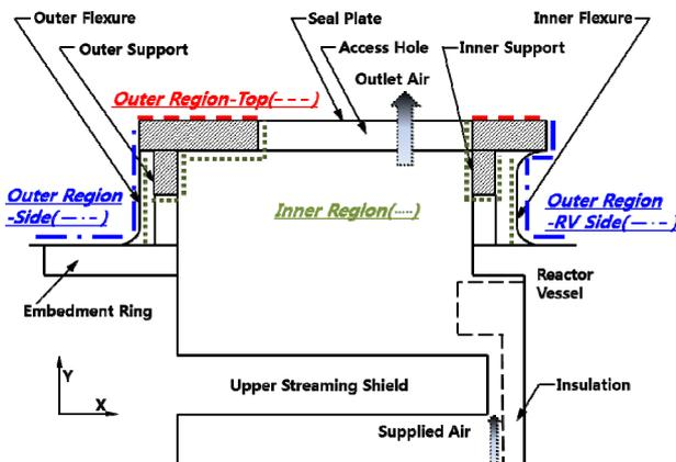
Fig. 1 Configuration at the Reactor Cavity
