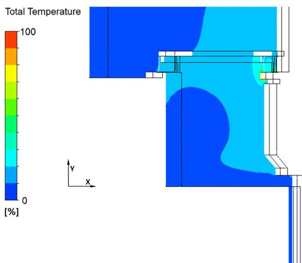
Fig. 2 Temperature Distribution at the Reactor Cavity (Cross-section via access hole)
