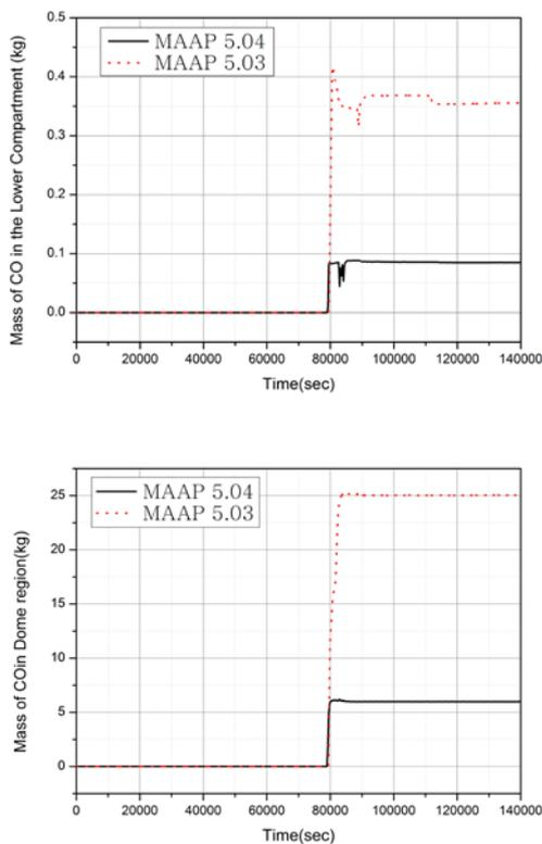
Fig. 2. Comparison of CO mass between results of MAAP 5.03 and MAAP 5.04 beta (top) lower compartment (bottom) dome
