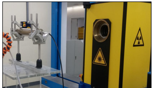
Fig. 3. Position of BF3 Detector at Gamma Source
