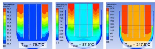
(a) Bare (b) Gallium flooding (c) Oil flooding
