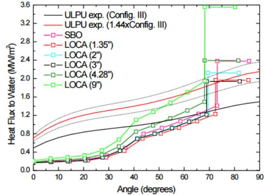
Fig. 1 Heat flux on the external surface of the RPV in various accident in APR 1400 [22]
