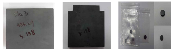
Fig. 1. Photos of SiC samples used for measuring thermal conductivity.
