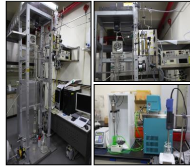
Fig. 2. Experimental apparatus (gelation column and carbon black powder dispersion equipment).
