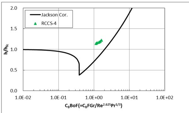
Fig. 11. Comparison of heat transfer coefficients with the Jackson correlation [11]
