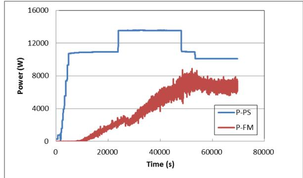
Fig. 4. Applied power (P-PS) and removed power (P-FM)
