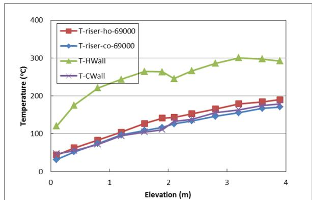
Fig. 5. Temperature distribution in test walls (t = 69,000 s)
