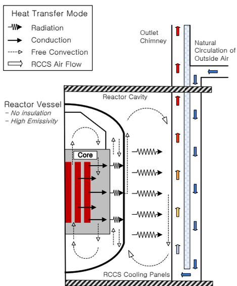
Fig. 1. Natural cooling phenomena in the air-cooled RCCS
