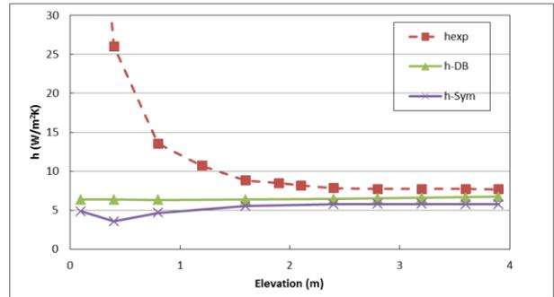
Fig. 9. Heat transfer coefficients along a riser ( $t = 69,000$  s)
