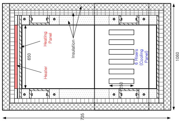
Fig. 3. Cross-sectional view of the NACEF test section
