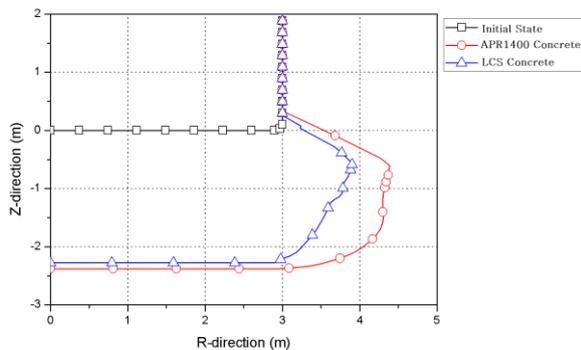
Fig. 3. Concrete Ablation from each Concrete Composition
