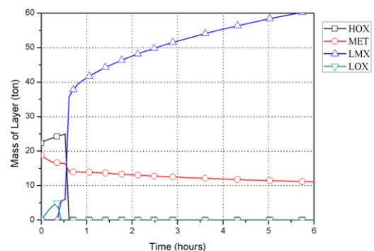
Fig. 1. Initial Layer Inversion of Metal and Oxide
