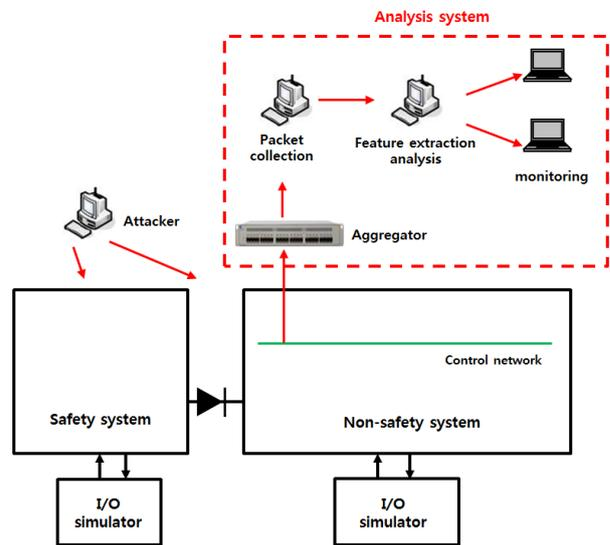
Fig. 1. Overall schematic of the cyber security test-bed
