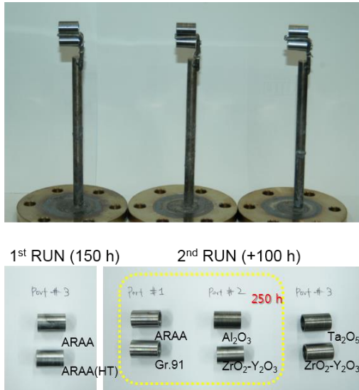
Fig. 2. Photographs of the fabricated specimens fixed to posts for the corrosion test (above) and specimens after the corrosion test (below).
