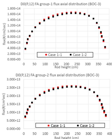
Fig. 4. Axial flux distribution at beginning of cycle
