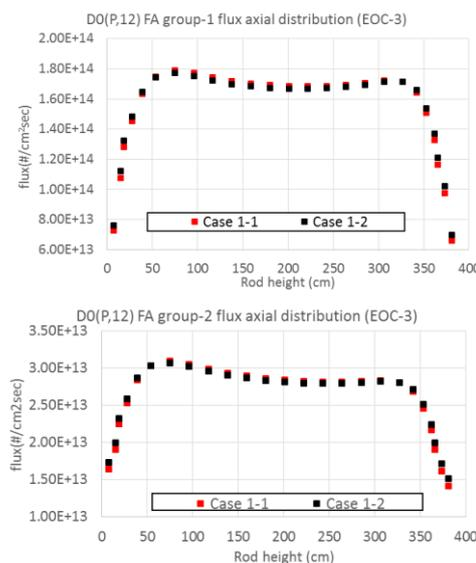
Fig. 5. Axial flux distribution at end of cycle
