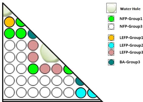
Fig. 10. B1 fuel assembly with grouping
