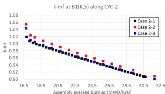
Fig. 6. k-inf curve of B1(K,5) assembly at CYC-2
