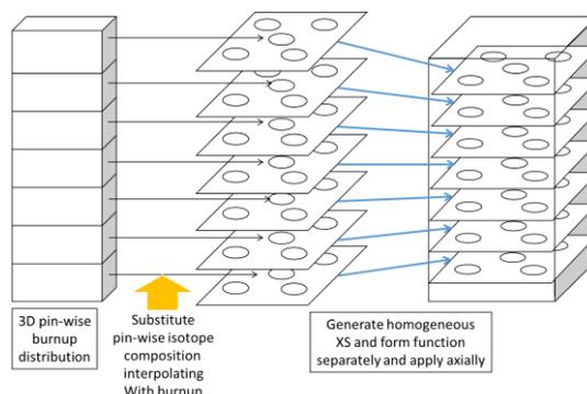
Fig. 2. Pin-wise composition retrieval technique with axial effect
