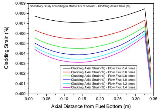
Fig. 8. Sensitivity analysis with change of coolant mass flux – cladding axial strain
