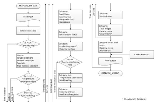
Fig. 1. Calculation flow diagram of FRAPCON-SFR.
