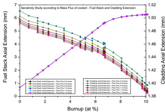
Fig. 6. Sensitivity analysis with change of coolant mass flux – fuel stack and cladding extension
