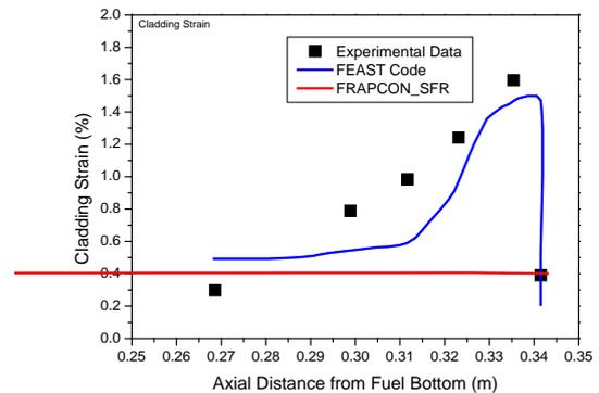
Fig. 4. Peak cladding strain of X447 data and code calculations
