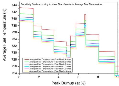
Fig. 5. Sensitivity analysis with change of coolant mass flux – average fuel temperature
