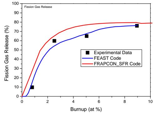
Fig. 3. Fission gas release behavior of X447 data and code calculations
