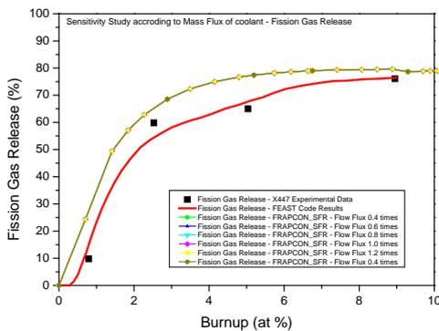
Fig. 7. Sensitivity analysis with change of coolant mass flux – fission gas release
