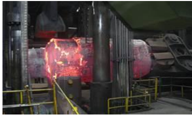
Figure 3 Appearance of prototype monoblock LP rotor shaft with \phi 2,800 mm at finishing forging stage.
