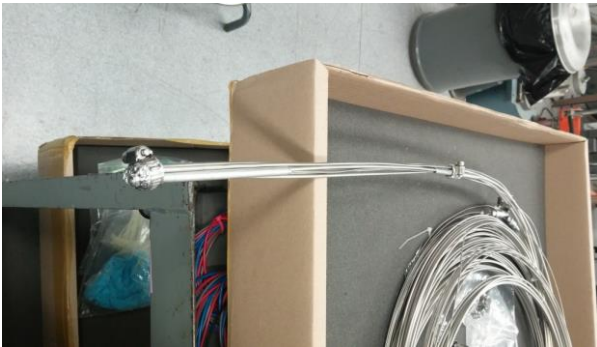
Fig. 3. The assembly of SPNDs
