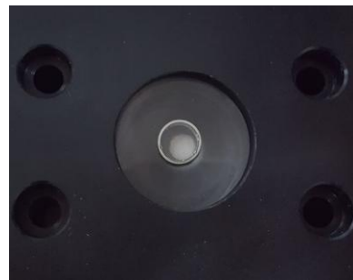
Fig. 1. Cross-sectioned test sample fixed to sample holder
