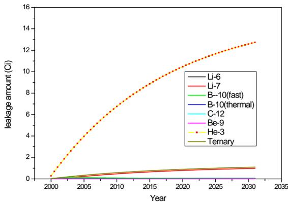
Fig. 6 Tritium leakage by the inventory – replacement
