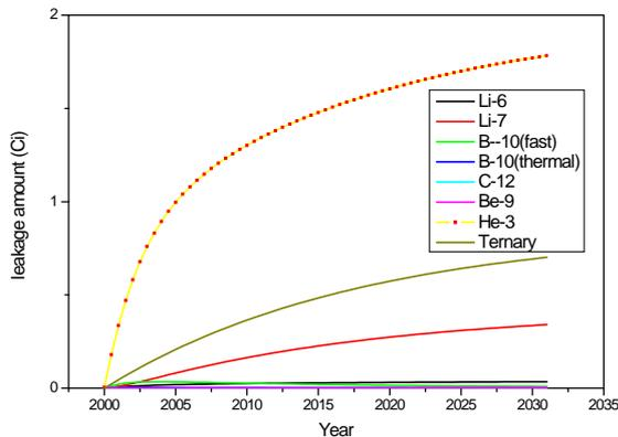
Fig. 7 Tritium leakage by the inventory – temperature effect
