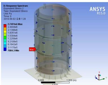
Fig. 4. Equivalent stress distribution of the buckles by spectrum analysis
