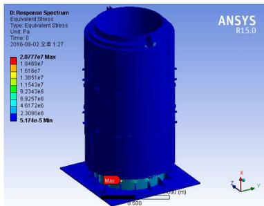
Fig. 3. Equivalent stress distribution of the test system by spectrum analysis
