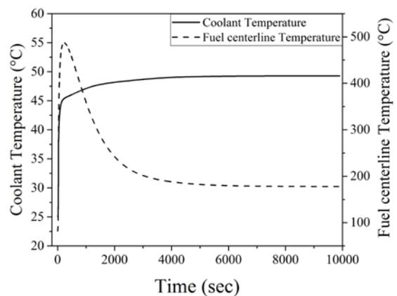
Fig 4. The average fuel centerline temperature and coolant temperature responses in the hottest fuel assembly.
