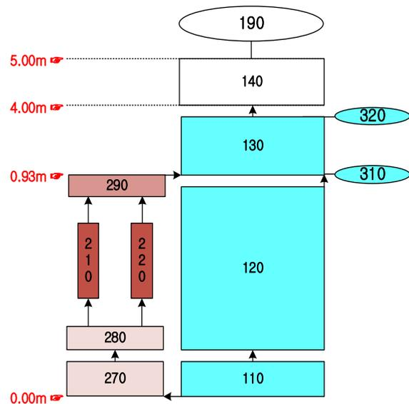
Fig 1. Nodal Diagram of Hybrid Low Power Research Reactor(H-LPRR)
