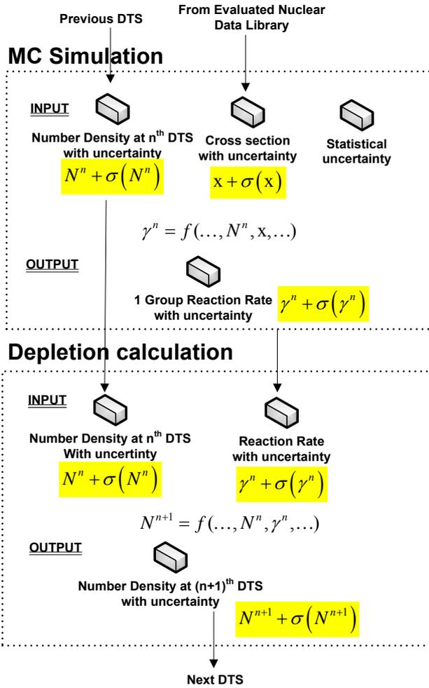
Fig. 5. Flowchart of uncertainty propagation procedure in MC depletion analysis by the SNU formulation
