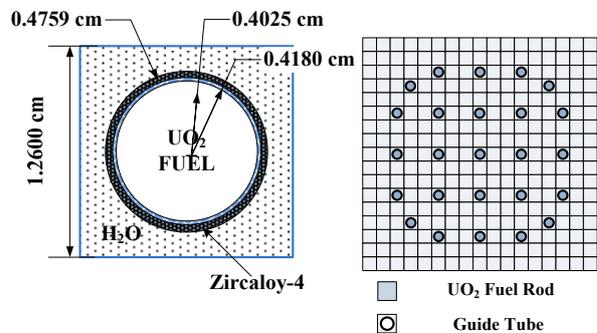
Fig. 1. Configuration of Pin Cell and FA Problem
