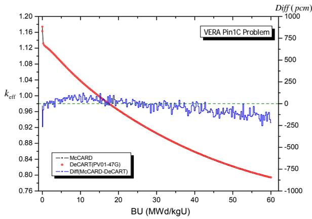
Fig. 2. Comparison of the evolutions of infinite multiplication factor and their discrepancies over burnup for VERA pin problem (242 DTS)
