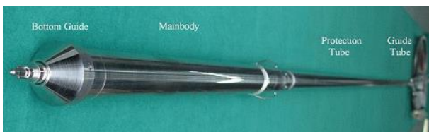
Fig. 1. The Instrumented Capsule for irradiation test in research reactor.
