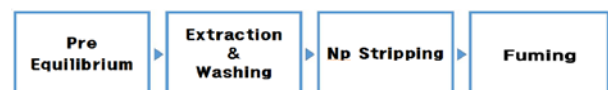
Fig 3. Flow diagram for milking of ^{239}\text{Np} from ^{243}\text{Am} by solvent extraction using Tri-n-octylamine
