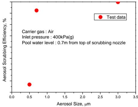
Fig. 4. Aerosol scrubbing efficiency against aerosol size (carrier gas : air, inlet pressure : 400kPa(g), pool water level : 0.7m from top of scrubbing nozzle)
