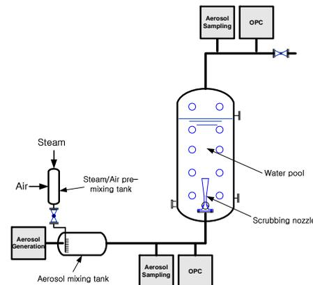
Fig. 2. Schematic of aerosol scrubbing test loop.
