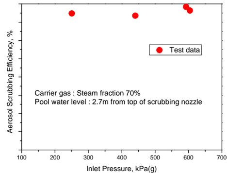
Fig. 7. Aerosol scrubbing efficiency against nozzle inlet pressure (carrier gas steam fraction : 70%, pool water level : 2.7m from top of scrubbing nozzle)
