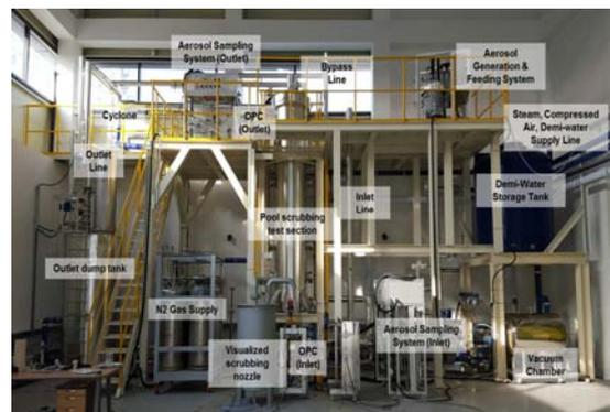
Fig. 3. Overview of aerosol scrubbing test loop
