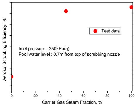
Fig. 5. Aerosol scrubbing efficiency against carrier gas steam fraction (inlet pressure : 250kPa(g), pool water level : 0.7m from top of scrubbing nozzle)
