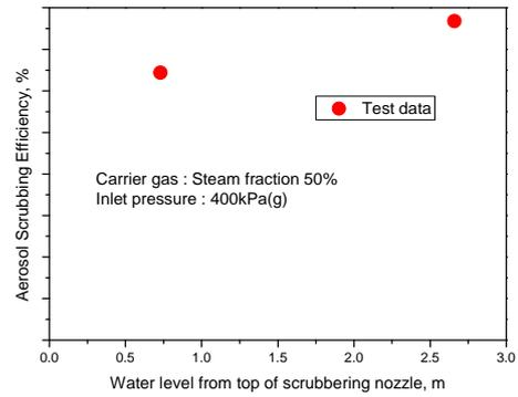
Fig. 6. Aerosol scrubbing efficiency against pool water level (carrier gas steam fraction : 50%, inlet pressure : 400kPa(g))
