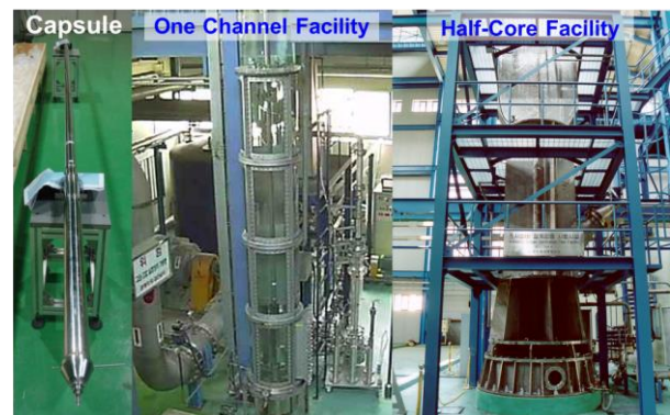
Fig. 1. An irradiation capsule and out-pile testing facilities at HANARO
