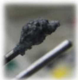
Fig. 3. Photograph of working and counter electrode with electrochemically deposited praseodymium.
