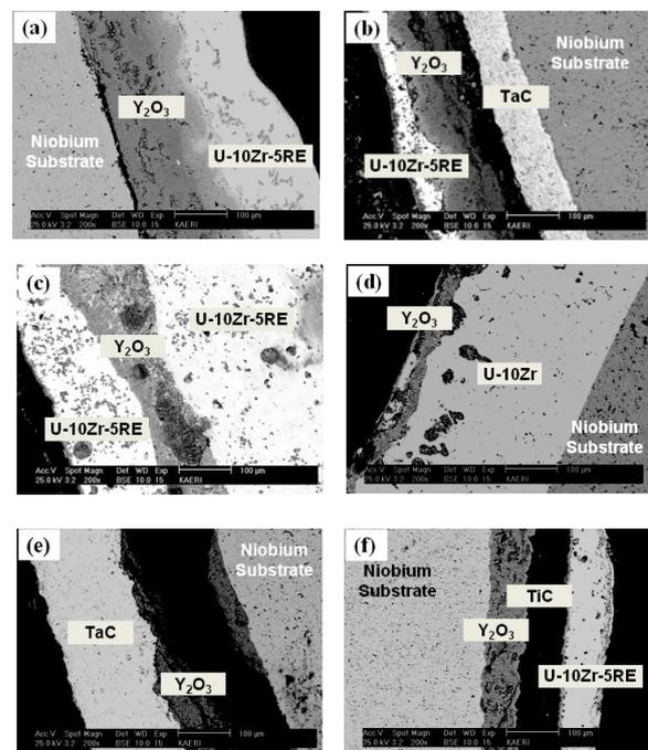
Fig. 1. Cross-sectional BSE micrographs showing the interface between U-10wt.%Zr-RE and coating layer after two cycles of dipping at 1600°C for 5 min: (a)  $Y_2O_3(150)$ , (b) TaC(50)- $Y_2O_3(100)$ , (c)  $Y_2O_3(50)$ -TaC(100), (d)  $Y_2O_3(50)$ -TiC(100), (e)  $Y_2O_3(100)$ -TaC(100)- $Y_2O_3(100)$ , and (f)  $Y_2O_3(100)$ -TiC(100)- $Y_2O_3(100)$ .
