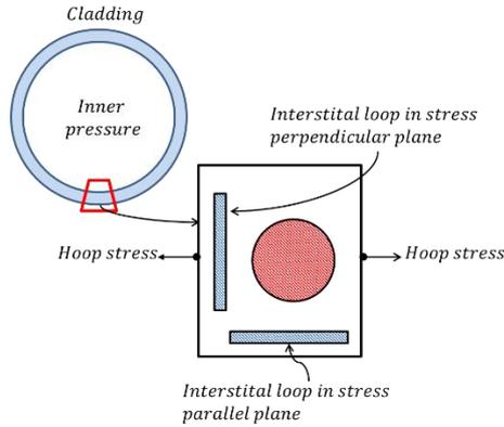
Fig. 1. Schematic of stress preferential induced nucleation.
