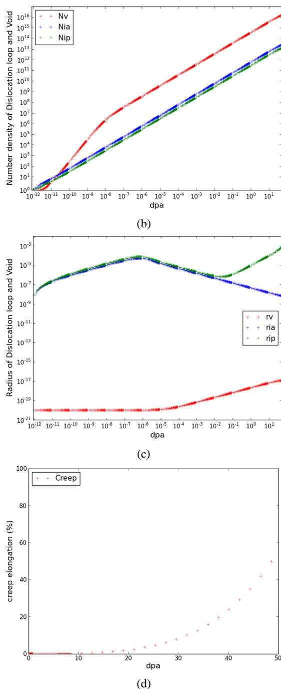
Fig.2. (a) defect concentration of point defect in iron matrix; (b) dislocation loop and void number density; (c) dislocation loop and void average radius; (d) irradiation creep elongation
