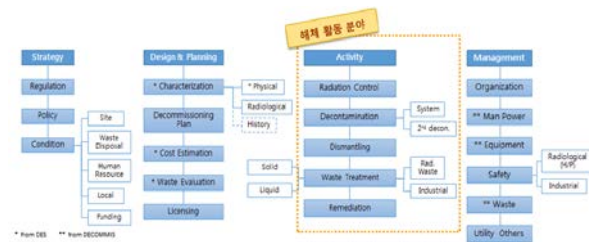
Fig. 1. Group items that should be managed for the requirements of the whole life cycle of the decommissioning
