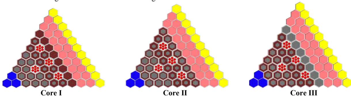
Fig. 1. Configuration of the reference core (1/6)
