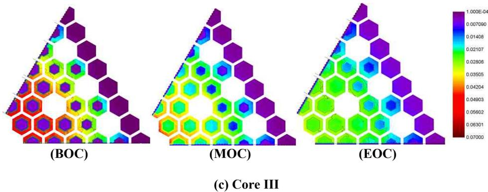
Fig. 3. Comparison of the pin-wise power distributions at BOC, MOC, and EOC
