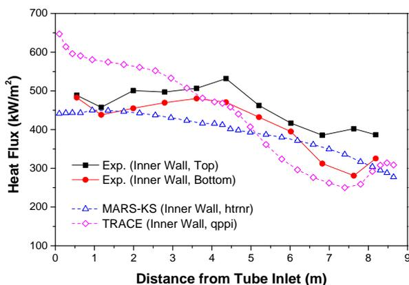
Fig. 3 Heat fluxes along the PCHX length
