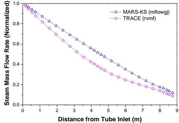
Fig. 6 Mass flow rate of steam along the PCHX length
