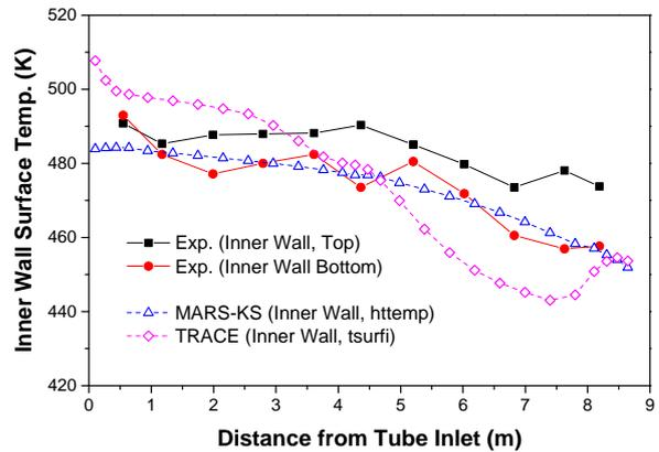
Fig. 4 Inner wall surface temperature along the PCHX length
