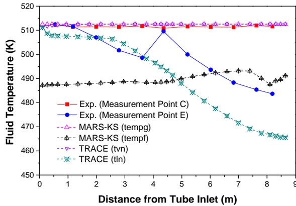
Fig. 5 Fluid temperature along the PCHX length
