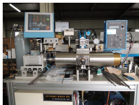
Fig. 2. Photograph of the GTAW system for end plug welding.
