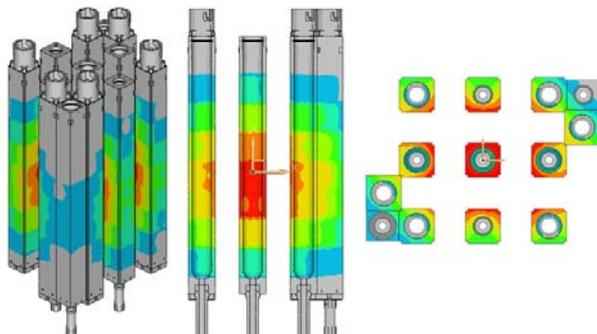
Figure 3 Neutron Fluence in the Finite Element Model
