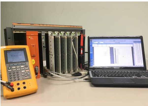
Fig. 4. Equipment Setting for Using the Calibration Tool
