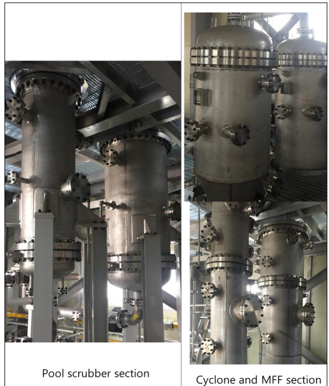
Fig.2. The 1:1 height, reduced diameter scale CFVS facility ARIEL to determine aerosol and iodine retention
