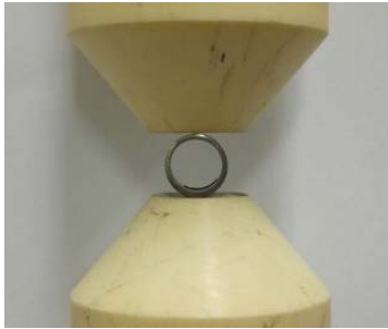
Fig. 2. Ring compression device and specimen.
