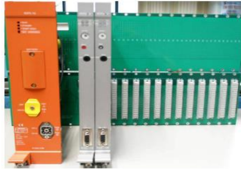
Fig. 1. Configuration of redundant processor module of POSAFE-Q [2].
