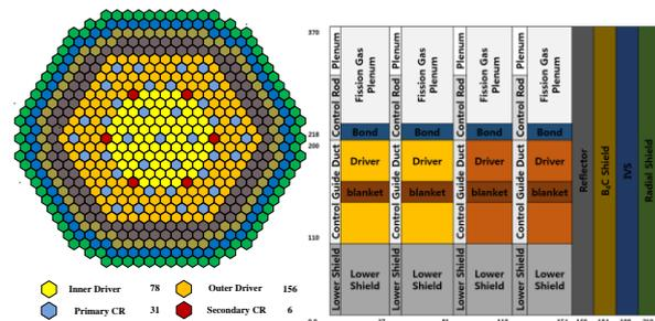
Fig. 1. Configuration of the SFR burner core
