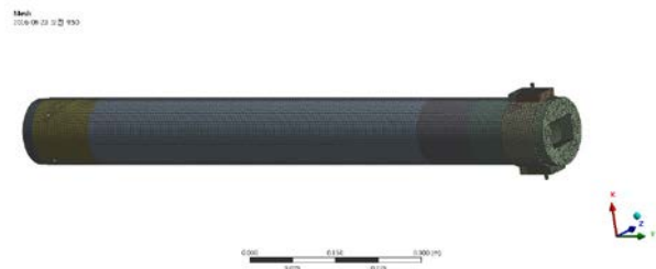
Fig. 1. Finite element model for damaged fuel canister
